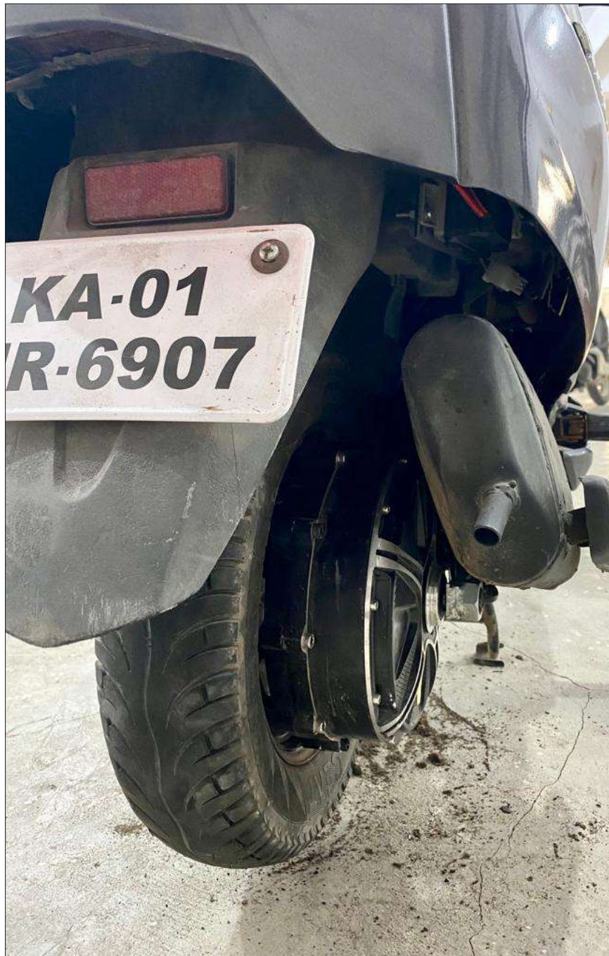
Petrol two-wheeler converted to Hybrid by retrofitting
