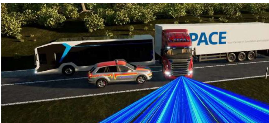
Figure 2 Full braking with a lower coefficient of friction: A much more critical situation arises, as the lower coefficient of friction lengthens the braking distance and completely changes the movement behavior of the truck-trailer combination. The truck protrudes into the oncoming lane.
