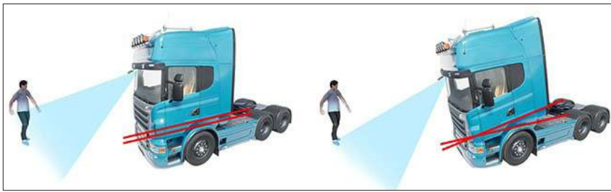
Figure 3 The pitch angle changes the view of the detected obstacle. A strong pitch angle even leads to the obstacle only being partially within the FoV of the sensor, which results in a more difficult object detection (perception).
