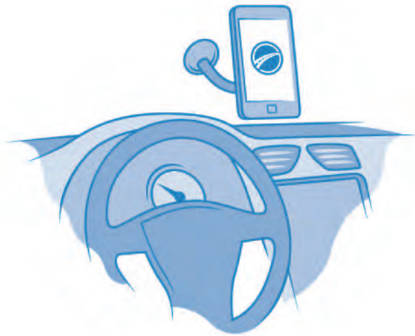
Fig. 2. Typical wind-shield mounting of the smartphone running an insurance telematics application (Courtesy: If P&C). The mounting supports smartphone based vision systems for smartphone-based looking in and looking out of a vehicle using the back and front mounted cameras, respectively; refer to e.g., [6].
